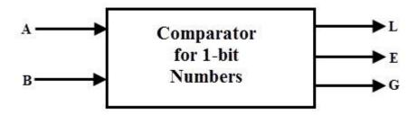
The truth table for the single bit comparator is given below. When A0 B0 = 00 & 11, both inputs are equal, therefore A=B output will be high. When A0 B0 = 01, B is more than A and hence AB is active.
